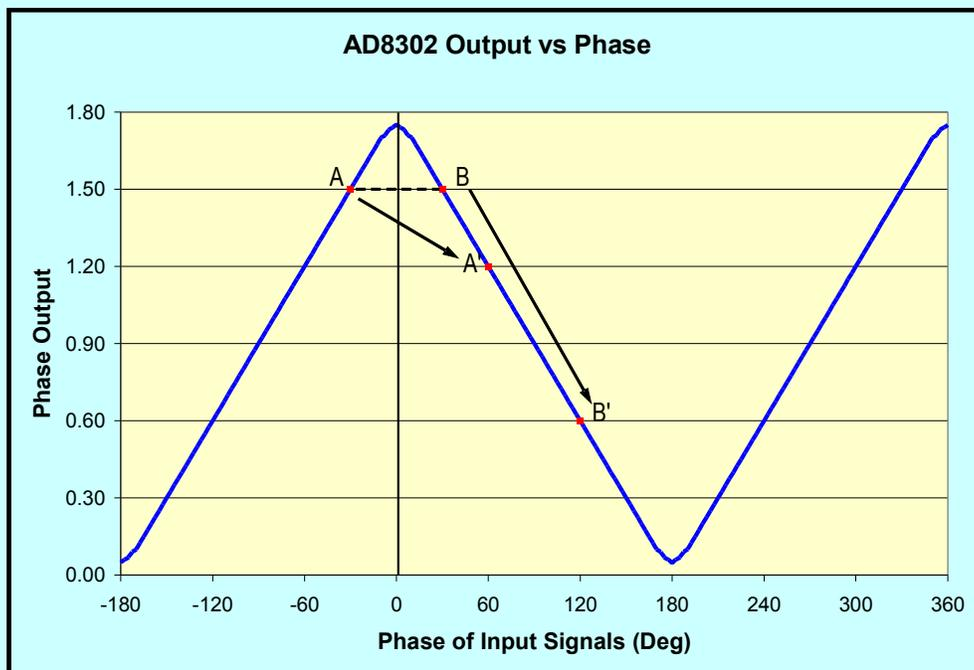
**Figure 1—AD8302 Output vs. Signal Input Phase**
