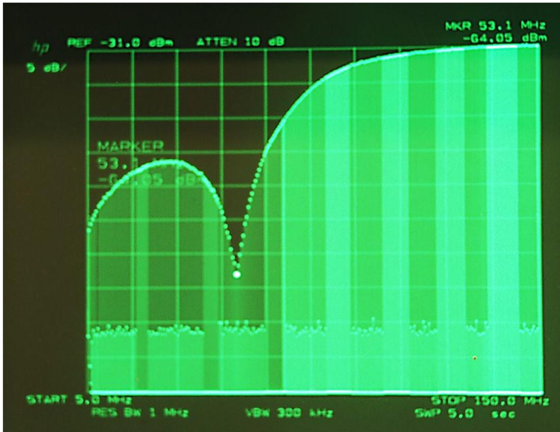
**Figure 8—Swept return loss of an LC lowpass filter. The spectrum analyzer reference level was adjusted so the bridge output with an open DUT was at the top of the grid. Return loss is the distance between the top and a point on the graph, based on 5 db per vertical division. The dip measures return loss of 33 db.**
