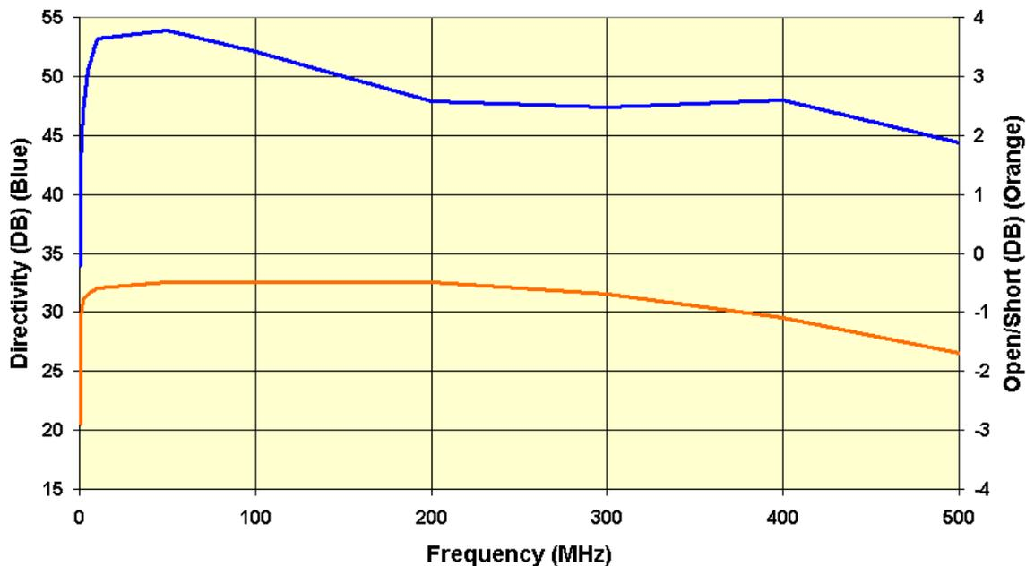
**Figure 4—Parallel Line Bridge Performance For Manual Measurements**
