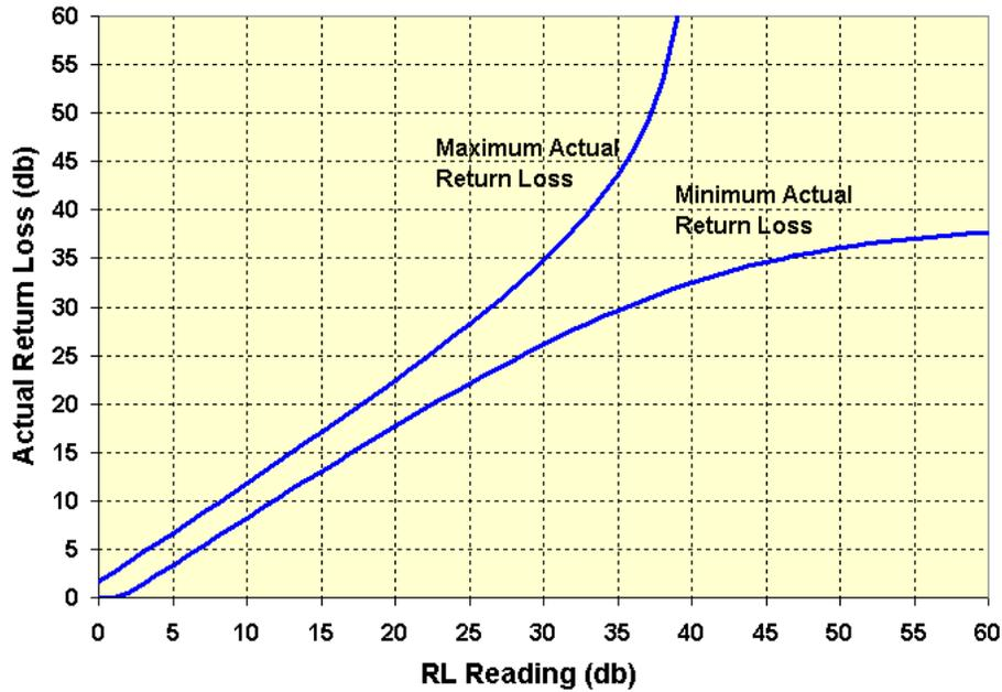
**Figure 6—Total error for directivity=40 db
