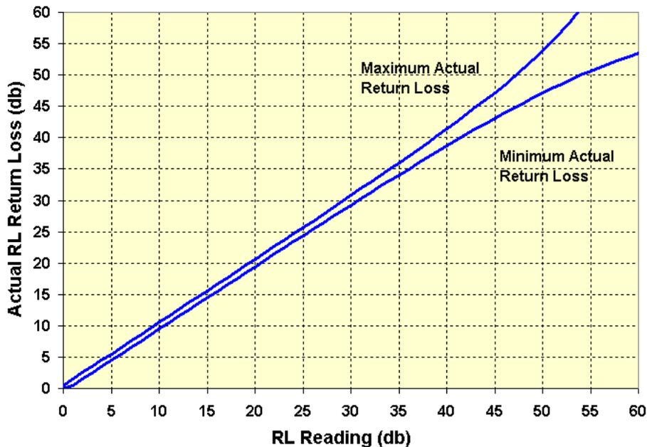
**Figure 10—Total error for directivity=60 db
