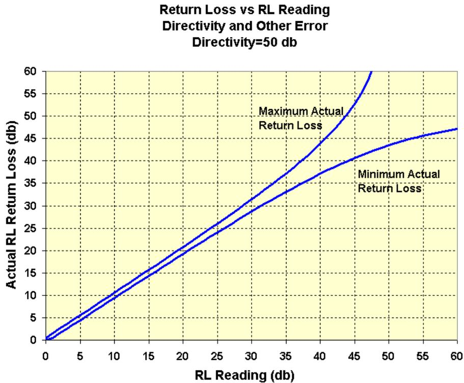
**Figure 7—Total error for directivity=50 db**
