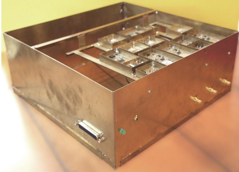
Figure 2—View of the back and left side. Parallel connector is on back; a separate power connector will be added. Side holds output connectors for DDS1, DDS2 and PLO3.
