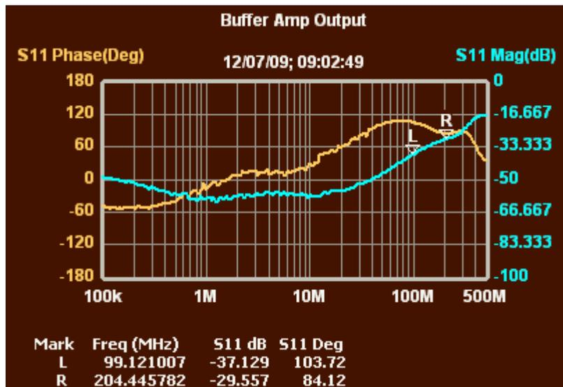
**Figure 3—Output Return Loss of Buffer Op Amp**
