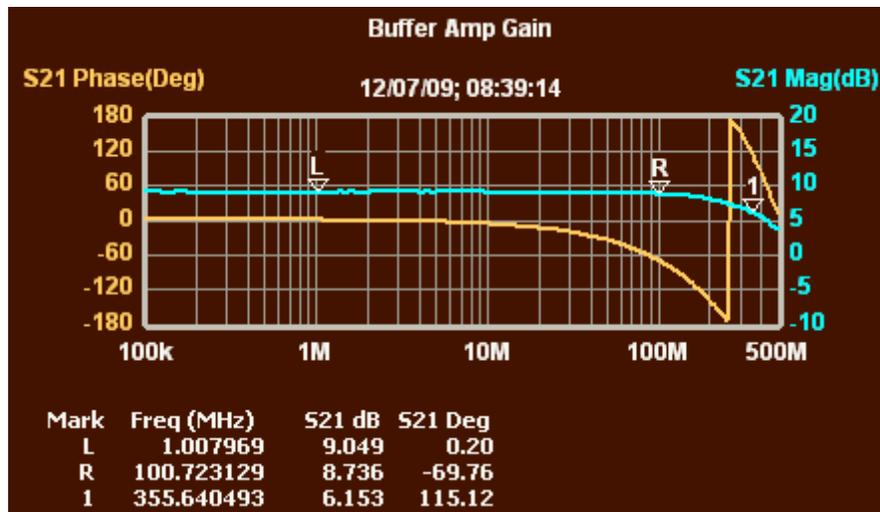
Figure 1—Gain of Buffer Op Amp
