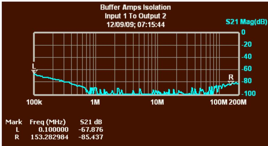
Figure 4—Isolation between amps
