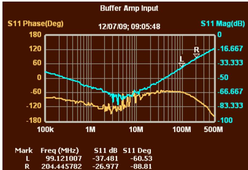
**Figure 2—Input Return Loss of Buffer Op Amp**
