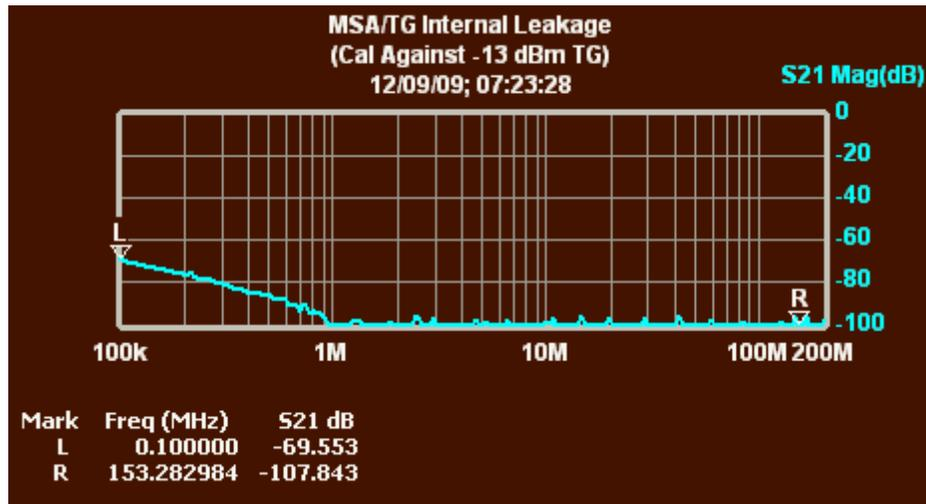
**Figure 6—MSA internal leakage when using TG**
