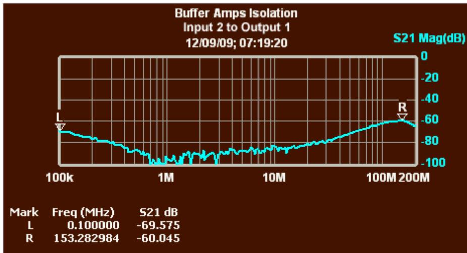
Figure 5—Isolation with the amps reversed
