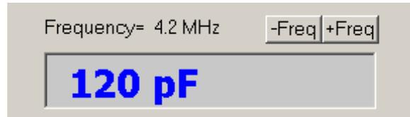
3. Click on the –Freq button to get the measurement at the next lower frequency, which will actually differ slightly from 120 pF. At low frequencies, the impedance of the capacitor becomes very high, which is difficult for the Shunt fixture to measure precisely. High impedances in shunt allow almost all the signal to pass by, and small changes in the impedance have very little impact on the transmitted signal. In the simulation, those small changes result from rounding errors.
