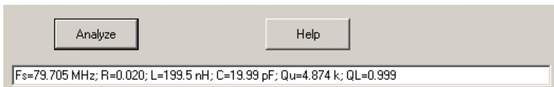
The values will not exactly match the simulated values, because an infinite-resolution scan would be required to perfectly identify the resonance and -3 dB points.
