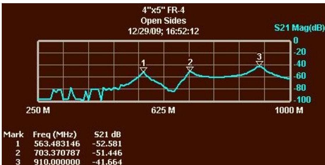
Figure 4—Transmission of FR-4 from corner to corner
