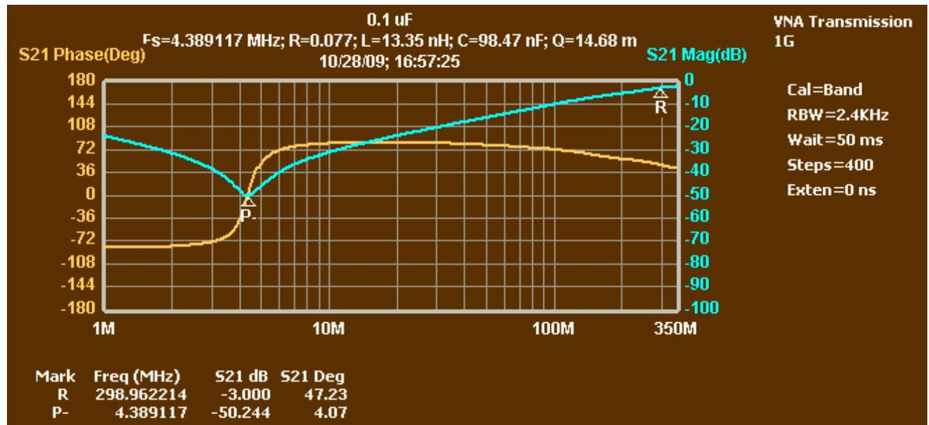
Figure 5—0.1 uF capacitor, measured as 98.5 nF
