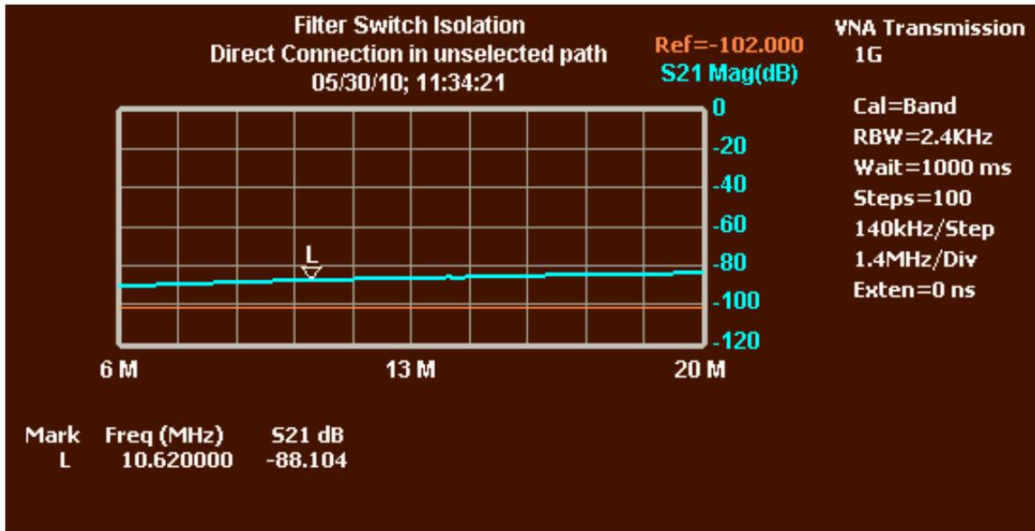
**Figure 3—Path 3 is direct connection**
