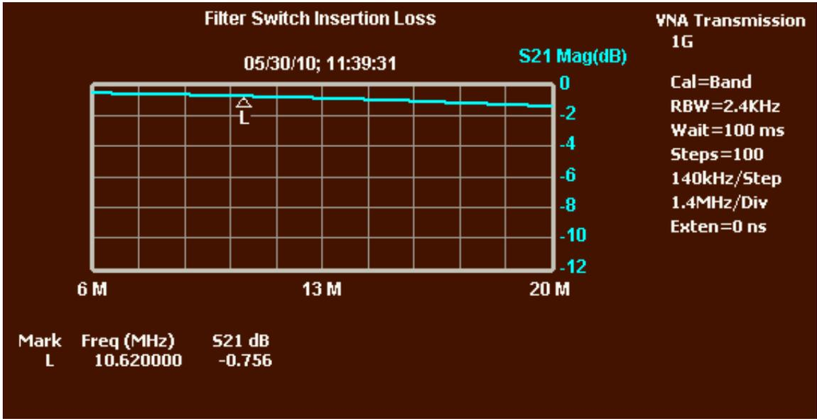
**Figure 5—Insertion loss**
